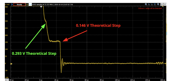
Fig. 9: -3.00 V input oscilloscope trace with not sharp steps above n=1.
